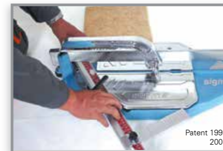
Metric bar with angle and measurement, always close to operator
