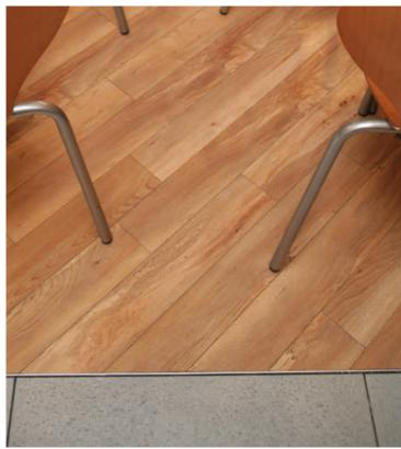
PROCARPET ACC is a profile in stainless steel 304/1.4301-V2A used for joining two floors of differing thickness and in particular for joining a tiled or parquet floor to wall-to-wall carpeting, making a perfect join thanks to the vertical part of less than 4 mm. In addition to completely protecting the edge of the higher floor, this particularly sturdy profile withstands high loads and supports the frequent passage of manual trolleys, vehicles and intense pedestrian traffic.
