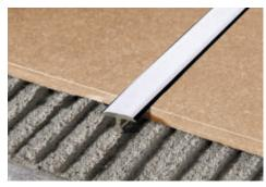
1. Choose "PROCOVER 1045 ALL" in the desired finish considering a side lap of 2/3 mm. 2. Fill the gap with single-pack silicone or with the adhesive used for laying the floor. 3. Bury the profile into the adhesive, making sure that both side laps of the profile rest on the coverings to be joined.
