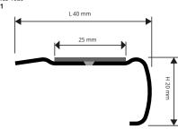
BRUSHED STAINLESS STEEL AISI 304/1.4301-V2A with protective film bar length 2,7 lm - pack. 20 Pcs - 54 lm
