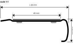
BRUSHED STAINLESS STEEL AISI 304/1.4301-V2A with protective film bar length 2,7 lm - pack. 20 Pcs - 54 lm
