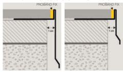
1. Choose "PROTERRACE PCG" according to the tile thickness. 2. Fix the external corners to the screed with nails taking care to separate them at least 1 cm from it. 3. Cut "PROTERRACE PCG" to the desired length. Lay the profile and fix it with nails. Connect it with the corners using the junctions. 4. Apply the desired waterproofing system. 5. Lay the tiles, leaving about 5 mm between tiles and profile. 6. Seal the space between tiles and profile with PROBAND FIX (P.186).
