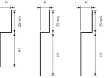
**PROSHOWER PROFILE WALL** Profile in satin-finish stainless steel AISI 304 / 1.4301 – V2A. It is suitable to cover and decorate the visible part of wall beside the shower tray in case of floor level showers with a slope of 2%.
