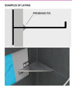
Choose "PROSHELF" according to the desired shape and size. 2. apply the adhesive on the support where the shelf will be installed. 3. Press the anchoring flap into the adhesive;
