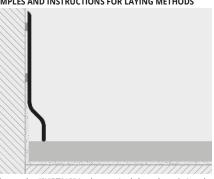
1. Choose the "SKIRTING" in the required the colour. 2. Lay the "SKIRTING" using quick-setting acrylic silicone, mastic or bostik, suitable for gluing flexible PVC onto mortar-plaster-accessorised walls, etc. or fix with screws/nails.
