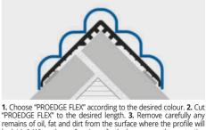
be laid. **4.** When the surface is perfectly dry, remove the protective film (version with adhesive), place correctly the profile and press it without hitting / apply the silicone on the surface where the profile will be laid (version without adhesive) and press it without hitting.
