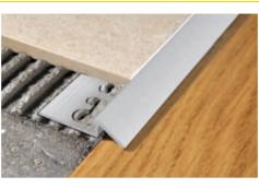
1. Choose the profile with the required finish. 2. Fill the profile cavity with adhesive and apply the adhesive onto the area of application. 3. Lay the "PROSLIDER KL ALL". 4. Align it flush with the floor/covering. 5. Use the adhesive to seal any empty interstices.
