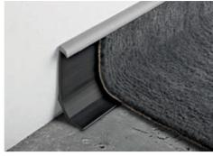
EXAMPLES AND INSTRUCTIONS FOR LAYING METHODS 1. Select the "SKIRTING COVECAP" of the desired color and height. 2. Using a utility knife cut the "SKIRTING COVECAP" to the desired length.  $\ensuremath{\mathbf{3}}$  . Apply the proper adhesive or glue/mastic and install the profile
