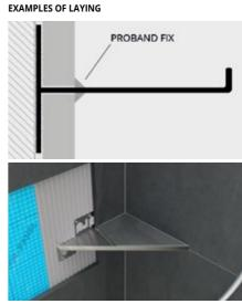
1. Choose "PROSHELF" according to the desired shape and size. 2. apply the adhesive on the support where the shelf will be installed. 3. Press the anchoring flap into the adhesive; 4. Lay the tiles taking care to align them with the shelf. Immediately remove adhesive residues from the surface of the shelf. 5. Carefully seal the joints between the shelf and tiles with PROBAND FIX to avoid water stagnation. Remove any grout residue from the shelf surface.
