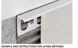
1. Choose "PROTERMINAL" according to the tile thickness and desired colour. 2. Cut "PROTERMINAL" to the desired length and apply the adhesive on the support where the profile will be laid. **3.** Press the anchoring flange of "PROTERMINAL" into the adhesive. **4.** Lay the tiles, aligning them with the profile leaving a 2 mm joint. 5. Fill the joints between the profile and the tiles with grout, in order to avoid water stagnation.
