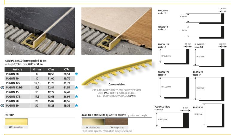
**PROLEVIGAL** are separating profiles used to create the technical joint in the special types of pavements such as marble- Venice- palladium ones, that must be smoothed after their laying process. The particular "L" shape with the cut/drilled base and 2,5 mm thick vertical edge consent the perfect smoothing and constant thickness as well. Available in natural aluminium and natural brass, various thickness, as well in outlined/bent **PROLEVIGAL** CURVE AL versions.
