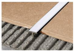
1. Choose "PROCOVER 1045 ALL" in the desired finish considering a side lap of 2/3 mm. 2. Fill the gap with single-pack silicone or with the adhesive used for laying the floor. 3. Bury the profile into the adhesive, making sure that both side laps of the profile rest on the
