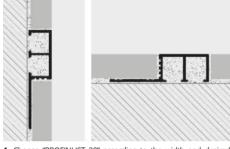
Choose "PROFINLIST 20" according to the width and desired finish. 2. Cut "PROFINLIST 20" to the desired length and apply the adhesive on the support where the profile will be laid. 3. Press the anchoring flange of "PROFINLIST 20" into the adhesive. 4. Lay the tiles, aligning them with the profile leaving a 2 mm joint. Remove immediately all remains of adhesive from the surface of the profile.
