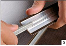
5) Keep the profile with the groove for insertion facing upwards and slot in the insert from the top downwards (if it does not slide easily, lubricate with water, silicone spray or vegetable oil).
