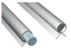
The **SNAP-ON PVC STRAND SHEATH** serves to cover/neutralise the reinforcement strands inside the prestressed beams; the sheath cancels out the stress that the strands transmit to the beam, thereby permitting the positive to be changed to left-handed moments. Available in various diameters and lengths.
