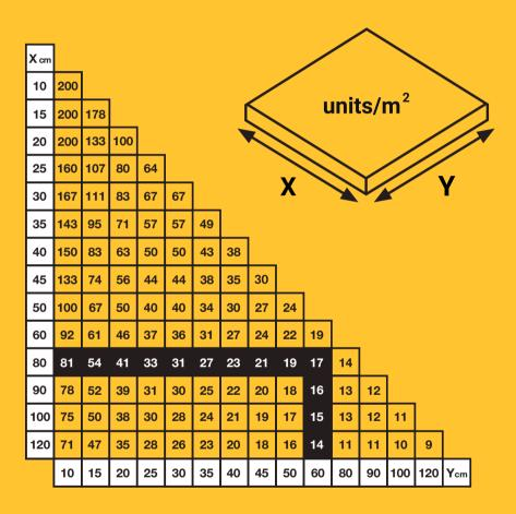
The required number of wedges is about one third of the number of clips. You can also order wedges in the amount that is required for the area that the tiler can lay per day.
