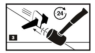
After glue has completely dried (about 24 hours), remove the system by hitting it with a mallet along the grout joint.
