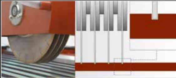
A selection of quality diamond discs for the processing of many different materials. From segmented discs for cutting building materials, tufa, granite and cement, to those for cutting, bevel and cutting simultaneously and grooving (creation of anti-slip channels) specifically designed for porcelain tiles. As well as discs for cutting ceramic: from the most delicate continual crown, to the "turbo" discs, an effective compromise between performance and quality of the cut.
