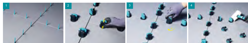
1 Place the level base under the tiles 10 cm from either end 2 Apply the fast clip cap to the level base 3 Close the cap and spin down to the required level to ensure no lippage 4 Remove the cap with BIHUI rubber mallet and open the cap simply for reuse
